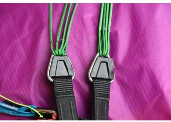
All BGD gliders are rigged from new with loops on the maillons of the C lines (and D lines if any) plus the stabi line. The loops are there so that they can be released to compensate for any shrinkage of the back lines as the glider gets older.
