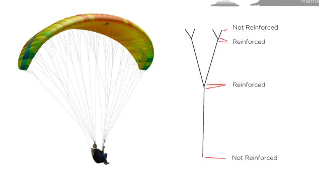
Unsheathed lines have an internal reinforcement at one end, marked with a yellow thread. This is the line junction end. The non-reinforced end is marked with a white thread and must be attached to the glider attachment point or maillon. Sheathed lines have no additional reinforcement and can be mounted in both directions.
