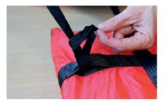
Connect the reserve handle to the reserve with a larksfoot knot to the middle loop on a side. Ensure that the strap is long enough to allow the plastic rods to be pulled out first.
