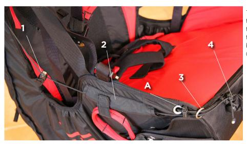
Thread the line through the pulley (1), then through the pastic tubing above the reserve handle (2). It then passes through the metal loop (3) before being tied securely to the speedbar, (4).
